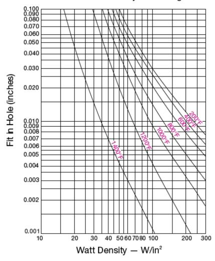
The graph shows the recommended maximum watt density for Tempco Hi-Density cartridge heaters at different operating temperatures and fit, when the heater is installed in an oxidized mild steel block. The thermocouple is located 1/2" from the heater. When heating other materials, the data needs to be extrapolated based on the thermal conductivity of the material. Consult Tempco with your requirements.
