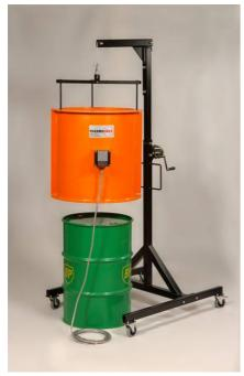
The sturdy steel frame is fitted with a braked winch with a safeworking-load significantly greater than either one Thermosafe Type A or two Type B heaters. Robust casters are fitted to the frame for full manoeuvrability and simple retaining bars and clips are used to secure and quick release the Thermosafe.
