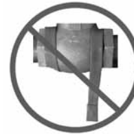
B.) Incorrect Installation: Heating tape hanging free from the surface
